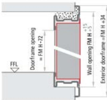
**Doors with internal lower threshold**
