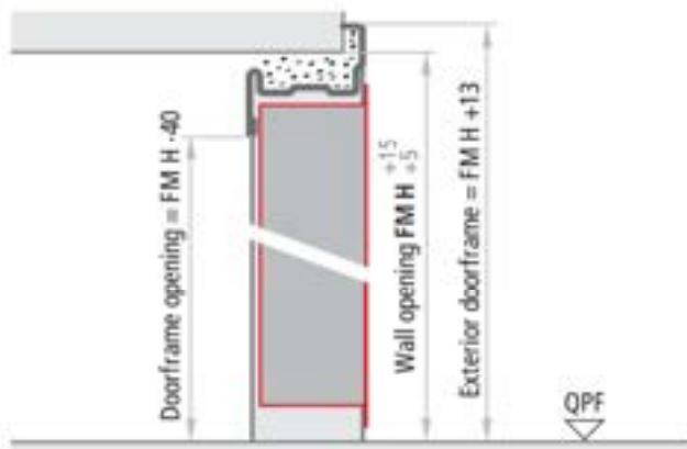
**Doors with internal and external lower threshold**
